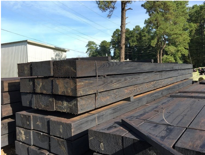
Figure 3: Timber treated with creosote (Reference Bayou Forest Products, 2017)
