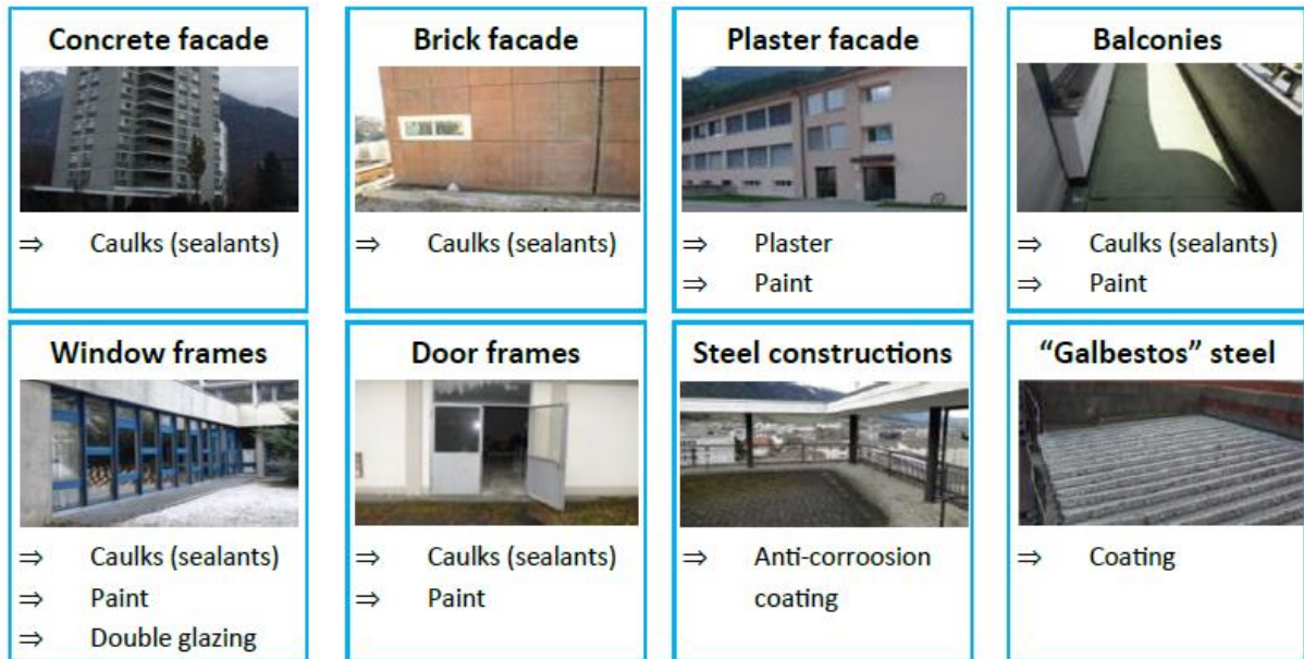
Figure 8: PCB in public and residential buildings – Outdoor environments
